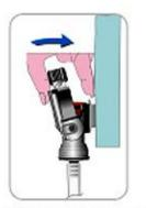
Place the tap inside the connector Push (pivot) to close the connector
